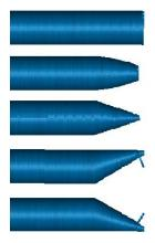
The different steil ends options. From top to bottom, Standard, Rounded, Sharp Point, 45 Cut Point, and 135 Cut Point.
